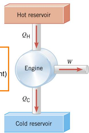
The **efficiency** of a heat engine is defined as the ratio of the work done to the input heat:
