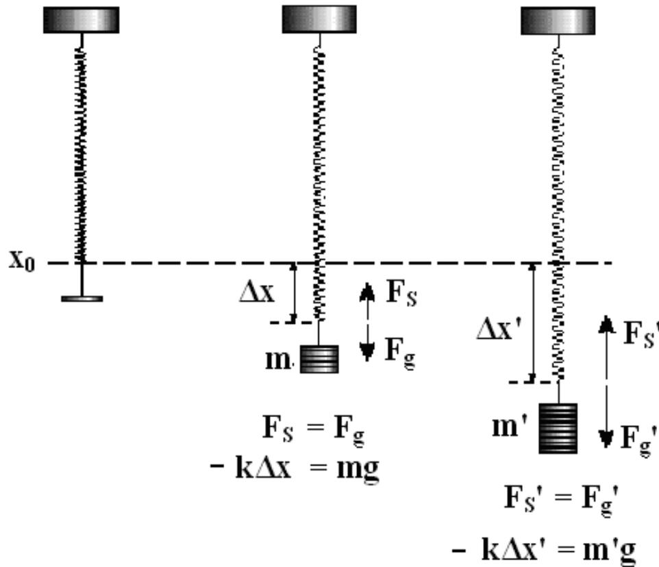
Figure 9.1: Force diagram of a spring in gravity.
