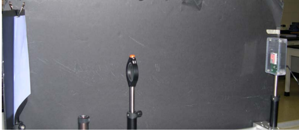
Figure 6.6: Optics bench with an object, a converging lens and a screen.
