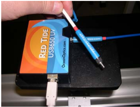
Figure 9.2: Digital spectrometer. Note the white USB cable and blue optical fiber.
