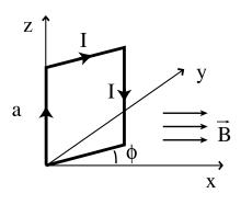
$$L(\phi, \dot{\phi}, q, \dot{q}) = \frac{1}{2} J \dot{\phi}^2 + \frac{1}{2} \mathcal{L} \dot{q}^2 - \dot{q} a^2 B \sin \phi.$$
