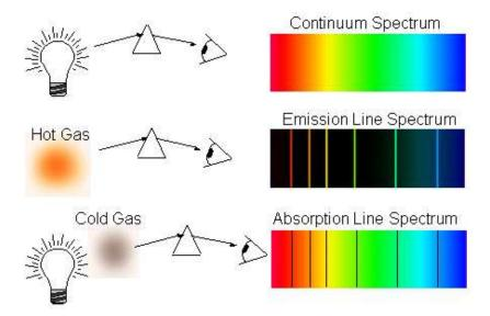
Figure 10.2: Examples of a continuous, an emission and an absorption spectrum with diagrams illustrating how the spectra were obtained.
