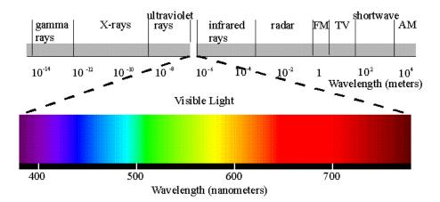
Figure 10.1: The electromagnetic spectrum with the visible light region blown up.
