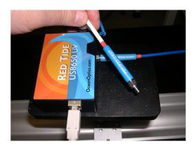
Figure 10.8: The digital spectrometer with a white USB cable and blue optical fiber plugged in.
