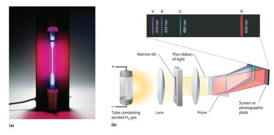
Figure 10.5: (a) A discharge tube containing hydrogen gas. (b) The experimental setup used to obtain an emission spectrum for hydrogen with the wavelengths of the 4 visible emission lines noted.
