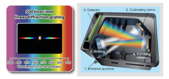
Figure 10.6: The diffraction grat-Figure 10.7: Schematic of how a digital ing.
