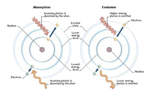
Figure 10.3: Model of an atom showing absorption and emission of photons.
