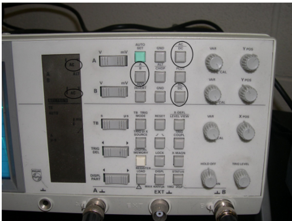
Figure 6.8: Front panel of the oscilloscope with the circled buttons indicating how to get channels A and B displayed simultaneously and in the AC coupling mode.
