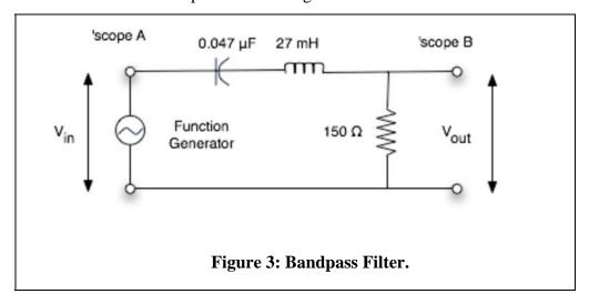
Use the DPO to show that the above is a bandpass filter. Print DPO displays showing input and output signals for frequencies below, within and above the transmitted band. Measure the resonance frequency. Compare with the resonance frequency of the low-pass
