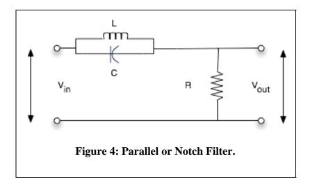
filter above. Measure the Q. Compare with the Q of the low-pass filter above.
