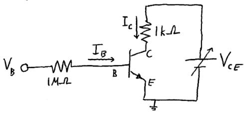
Labview steps the base current (by stepping V<sub>B</sub>). For each step, it plots I<sub>C</sub> versus V<sub>CE</sub>.
