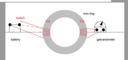
Close the switch  $\implies$  a temporary deflection of the galvanometer needle Open the switch  $\implies$  a temporary deflection of the galvanometer needle When the magnetic field CHANGES, there is an induced electric current in coil C2. But the induced current is a secondary effect. Electromagnetic Induction: When the magnetic field **B** changes (by closing or opening the switch) then there is an induced electric field **E** that curls around the change of **B**.
