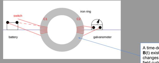
A time-dependent magnetic field **B**(t) exists around the ring. As it changes (in time) an electric field curls around the ring.
