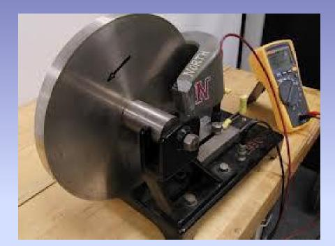
The first electric generator (Faraday, 1831); it creates a DC voltage from center to edge.
