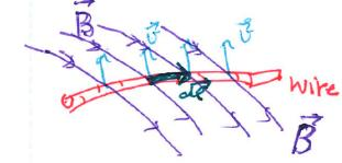
The EMF will drive a current I = EMF /R if the wire is part of a complete conducting circuit (*just like a battery would*).
