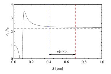
Index of refraction produced by UV natural frequency (Lorentz model)
