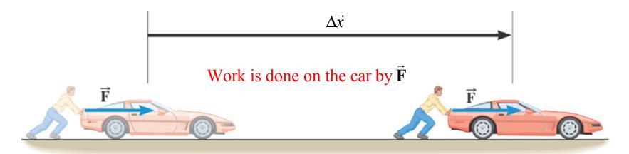
With only one force acting on the car  $(m_{Car})$ , the car must accelerate, and over the displacement  $\Delta \vec{x}$ , the speed of the car will increase.
