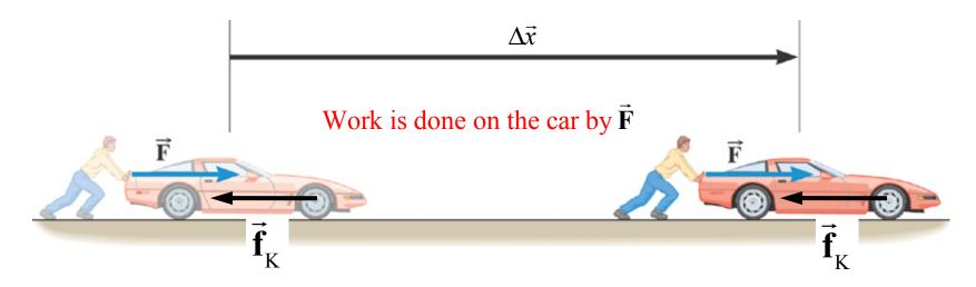
Also acting on the car is a kinetic friction force,  $\vec{\mathbf{f}}_K = -\vec{\mathbf{F}}$ . Net force on car must be ZERO, because the car does not accelerate!
