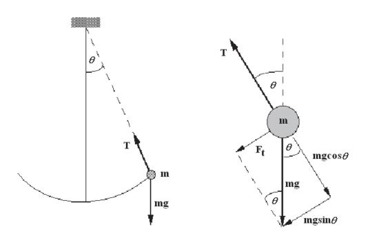
Figure 8.1: Force diagram of a pendulum
