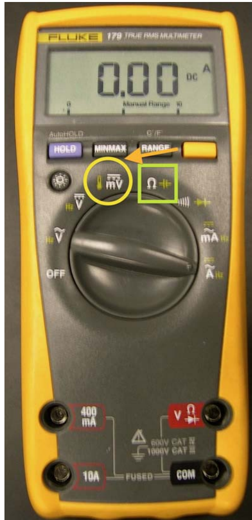
Figure 4.4: Digital multimeter with the green rectangle showing the setting for measuring resistance in ohms and the yellow circle showing the setting for measuring temperature in degrees Celsius. Notice that the latter setting will require the yellow button to be pushed (to the right of the RANGE button.)
