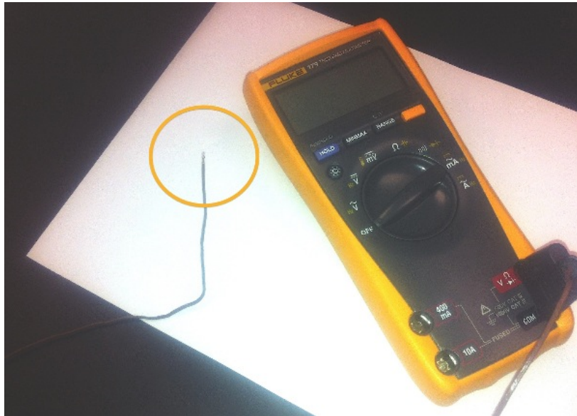
Figure 4.2: A thermocouple is a device that will respond to tiny changes in temperature (circled). It's attached to the multimeter.
