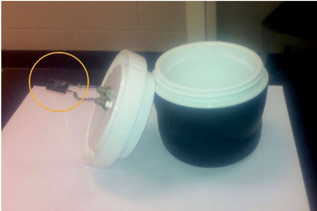
Figure 4.1: The calorimeter is a small “thermos bottle” with a screw-top lid in which a resistor is soldered (circled).
