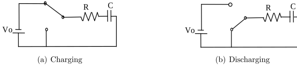
Figure 5.2: Schematics of charging and discharging a capacitor.
