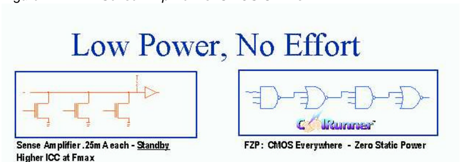
Figure 2.17 Sense Amplifier vs. CMOS CPLDs
