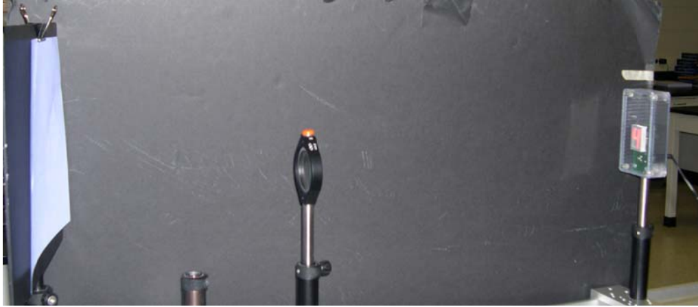
Figure 7.6: Optics bench with an object, a converging lens and a screen.
