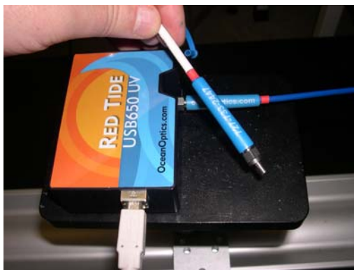
Figure 9.8: The digital spectrometer with a white USB cable and blue optical fiber plugged in.
