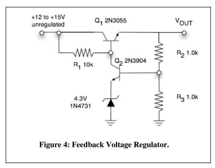
load conditions are variable. These can give output impedances less than an ohm and high stability against temperature variation. Figure 4 is a common example of a negative-feedback circuit. Transistor  $Q_1$  is normally conducting because of the bias current through  $R_1$ . When the output voltage reaches 10 volts,  $Q_2$  begins to conduct, shunting current away from the base of  $Q_1$  and preventing further rise of the output voltage. \*Explain why this happens.
