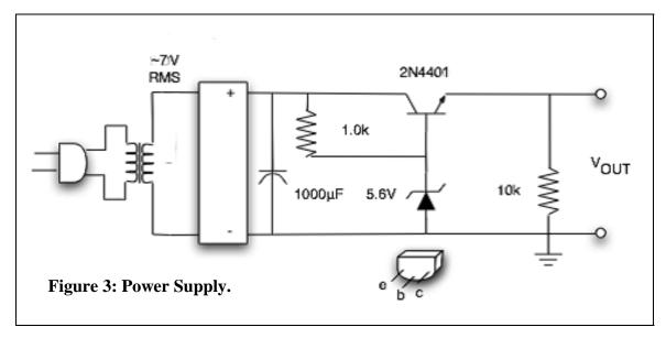
The rectangular box refers to the full-wave rectifier WL02F (alternatively RB152) and "NC" means no connections to the center tap on the transformer. The output should be about 5 volts. *Note*: A commercial full-wave rectifier bridge has 4 leads, two for AC
