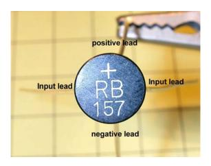
At times polarity of components may be marked with the length of the leads: a longer lead represents '+'.
