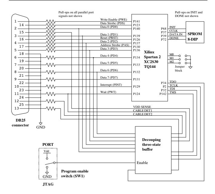
Figure 2. Parallel port and programming circuit schematic
