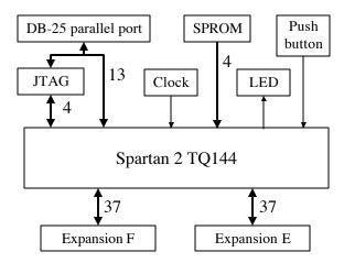
D2XL FPGA circuit block diagram
