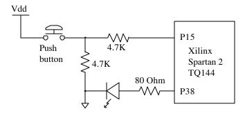
Figure 5. Pushbutton and LED detail
