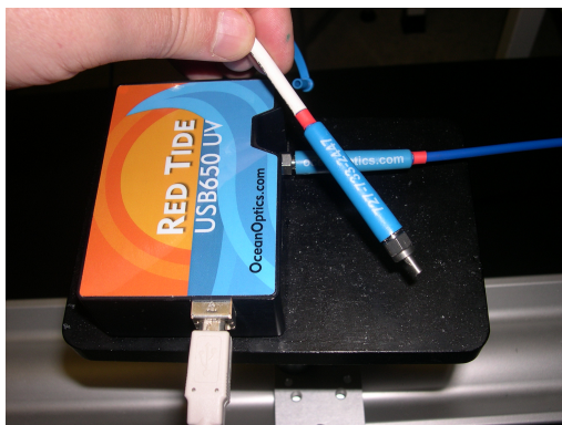
Figure 2.8: The digital spectrometer with a white USB cable and blue optical fiber plugged in.
