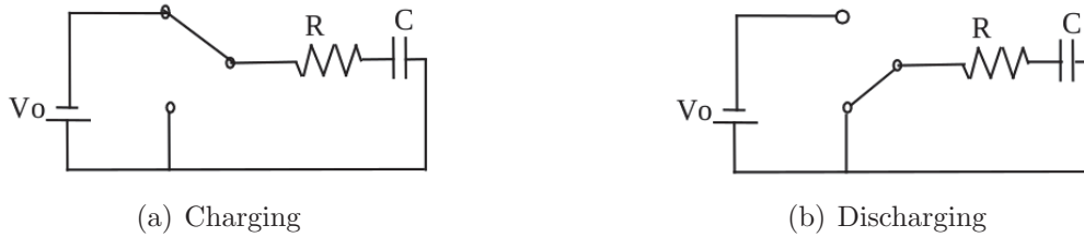
Figure 5.2: Schematics of charging and discharging a capacitor.
