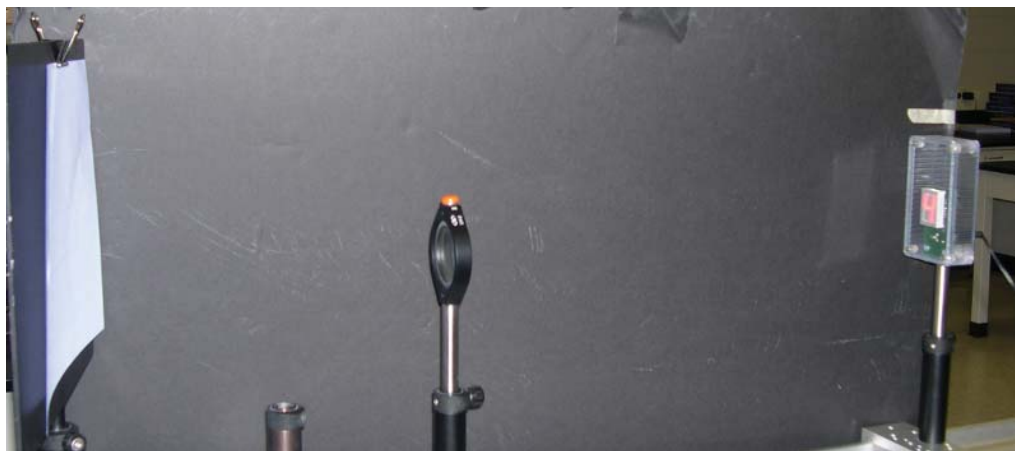
Figure 6.6: Optics bench with an object, a converging lens and a screen.
