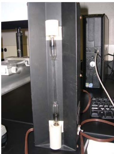
Figure 9.4: Gas discharge tube mounted in box.
