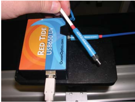
Figure 9.2: Digital spectrometer. Note the white USB cable and blue optical fiber.
