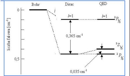
Lamb's shift: a subtle structure of the n=2 level in hydrogen according to Bohr's, Dirac's and QED with assumption Lamb's shift. The Lamb shift removes the degeneration due to quantum number *j*.
