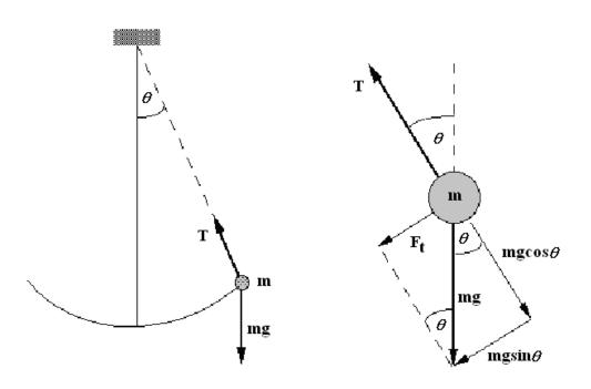
Figure 9.1: Force diagram of a pendulum
