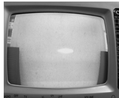
Figure 14c: Laser Beam with laser current well above threshold. An ND filter has been placed between laser and viewing screen, only laser light is visible
