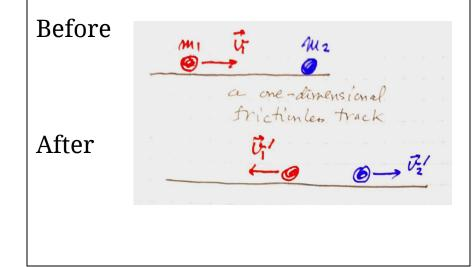
$M_1 U_1 = M_1 U_1' + M_2 U_2'$  $\frac{1}{2} m_1 v_1^2 = \frac{1}{2} m_1 v_1^2 + \frac{1}{2} m_2 v_2^2$ (elastic) Algebra to solve the quations =>  $U_1^{\prime} = \frac{m_1 - m_2}{m_1 + m_2} U_1^{\prime}$  and  $U_2^{\prime} = \frac{2m_1}{m_1 + m_2} U_1^{\prime}$
