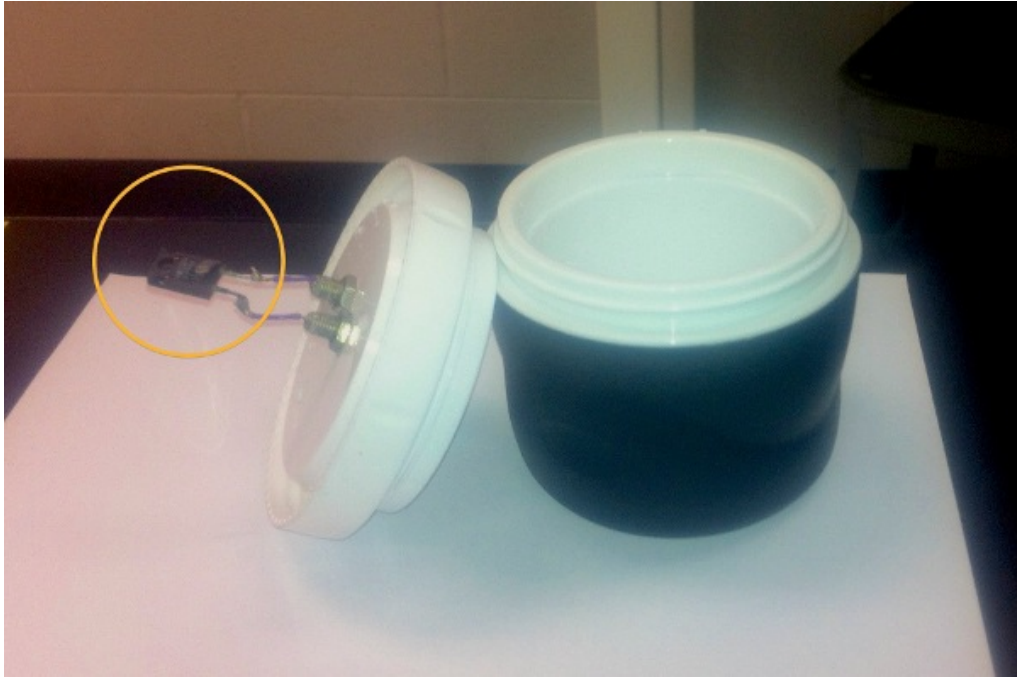
Figure 3.1: The calorimeter is a small “thermos bottle” with a screw-top lid in which a resistor is soldered (circled).
