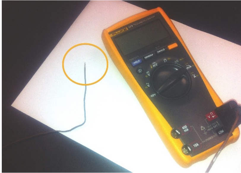
Figure 3.2: A thermocouple is a device that will respond to tiny changes in temperature (circled). It's attached to the multimeter.
