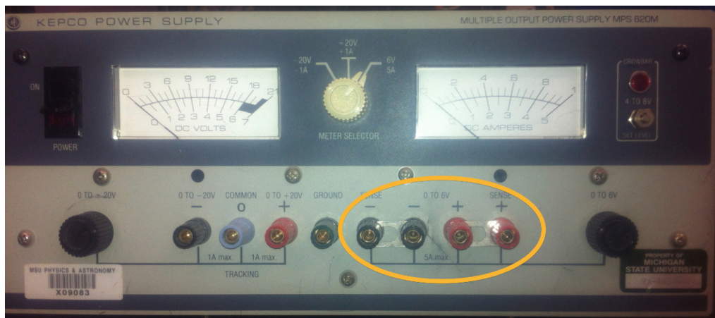
Figure 3.3: The power supply is a high-current device. We'll use the 6V and 5A maximum scales on the bottom of each of the windows. You connect to the resistor through the sockets on the top of the calorimeter and to the + and - "0 TO 6 V" connectors on the front (circled).
