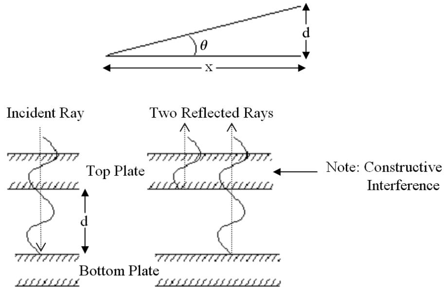
Because the beam reflected from the bottom of the film traverses the air gap twice, we see that the  $m^{\text{th}}$  bright fringe appears when
