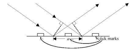
The condition for constructive interference:  $a(\cos \alpha - \cos \beta) = 0, \lambda, 2\lambda, ... = n\lambda$
