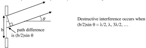
Now, each point source can be paired with one b/2 away. If one pair is out-of-phase, they will all be out-of-phase. Note that a minimum does not appear at  $\sin \theta = 0$ . The bright region arises from the undiffracted beam, i.e. the point sources away from the edges, which produce rays that arrive in-phase. Taking  $\sin \theta \approx \theta$ , we see that the minima occur at the angles shown below.
