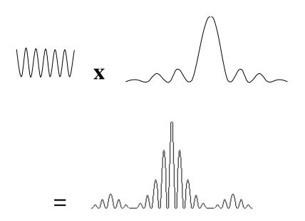
The pattern from multiple slits or a diffraction grating is calculated in a similar way.
