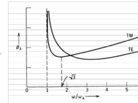
**Figure 8.6** Attenuation constant  $\beta_\lambda$  as a function of frequency for typical TE and TM modes. For TM modes the minimum attenuation occurs at  $\omega/\omega_\lambda = \sqrt{3}$ , regardless of cross-sectional shape.
