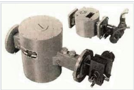
Two microwave cavities (left) from 1955, each attached by waveguide to a reflex klystron (right) a vacuum tube used to generate microwaves. The cavities serve as resonators (tank circuits) to determine the frequency of the oscillators
