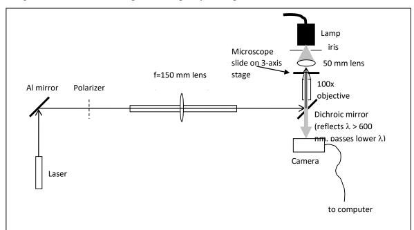
The figure below shows a completed setup of your experiment
