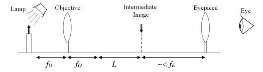
You may use the same lenses as before. As an object use selected location on the paper covered with text printed using the lab's printer.
