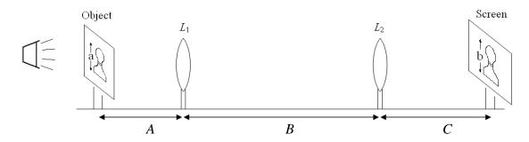
The image produced by the first lens  $L_1$  is at position  $s_1$  that can be found from the thin lens equation
