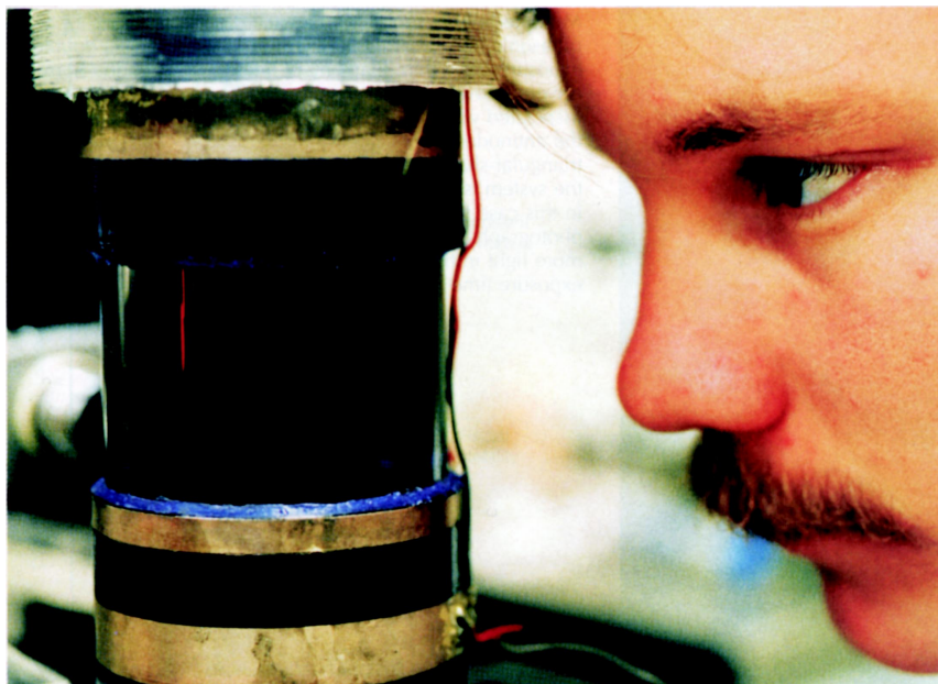
Acoustic cavitation and Sonoluminescence. This acoustic resonator consists of two transducers separated by a thin glass cylinder. Standing waves with frequencies from about 20 kHz to over 100 kHz and acoustic pressures up to about 3 bars can be generated in the liquid. If the acoustic-pressure amplitude is sufficiently large, many cavitation bubbles can be generated near the pressure anti nodes of the standing-wave system. If the pressure is considerably lower, it is possible to “acoustically levitate” individual gas bubbles, which under conditions described in the text can generate light each acoustic cycle. Graduate student Sean Cordry watches the blue sonoluminescence from such a bubble. The red streak is an artifact of the lighting. Figure 1
