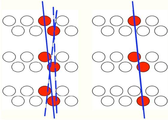
Fig. 3: Schematic view of 3 doublet layers. On the left, the doublet scheme is depicted, showing that beside from the correct track (solid blue line) other tracks (dashed blue lines) can trigger the same equation. With the singlet equation shown on the right, only the correct track fires the trigger
