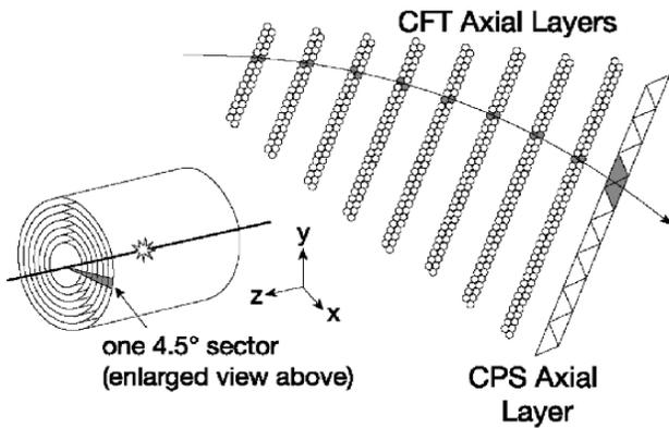
Fig.1: Schematic view of the axial part of the Central Fiber Tracker (CFT). It consists of 8 concentric doublet layers of scintillating fibers and a pre-shower detector (CPS) surrounding the interaction point. One of the 80 trigger sectors used by the CTT is shown with a hypothetical track overlaid.
