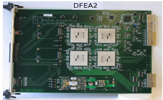
Fig. 4 DFEA2 board with 4 Xilinx Virtex 2 FPGAs in the center. Two boards were installed in a parallel chain in the DØ detector prior to full installation.
