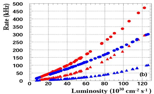
Fig. 2: Trigger rates for single (circle) and double (triangle) track triggers as a function of luminosity for doublet equations (red) and singlet equations (blue) for tracks with  $p_T > 3$  GeV.
