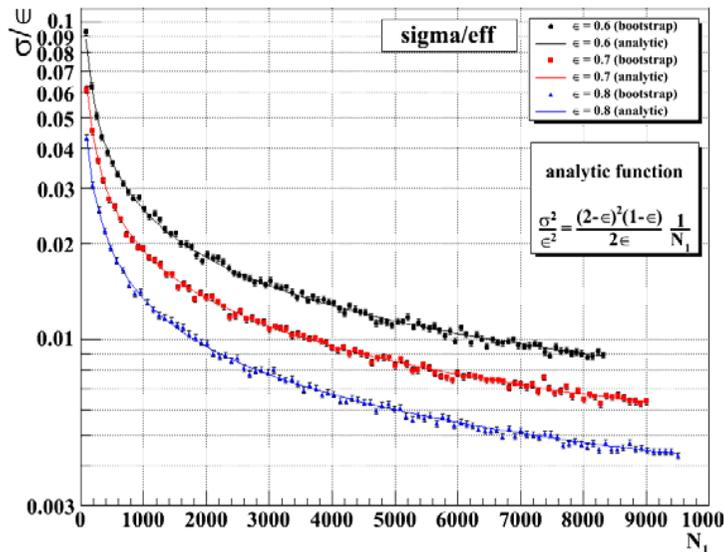
Assuming an HLT  $\mu 20$  trigger efficiency greater than 70 %, after 30 mins of DAQ the efficiency can be estimated with about 1-2 % statistical uncertainty
