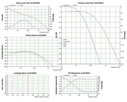
$\begin{array}{c} \text{SFX-524-CRN2} \\ \text{Exact frequency is 320.6296 MHz in and out.} \\ \text{ADF4111 design for 40M ref 320M out 200Hz Bw 67 deg mrgn 320kPFD.pll analysed at 08/26/13 14:52:24} \end{array}$
