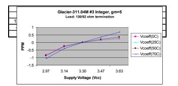
Voltage coefficient for the V777-311.04
