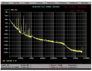
Typical Integrated jitter calculation
