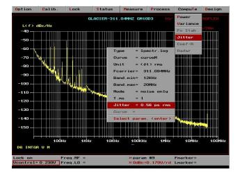
VCXO Using a X2 muliplier Typical phase noise
