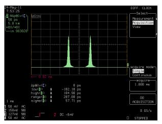
Analysis: The V777 jitter has a deterministic element to it due to the x2 multiplication scheme.
