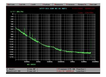
The typical integrated jitter for the VCXO above between 12KHz and 20 MHz is 0.100 ps rms
