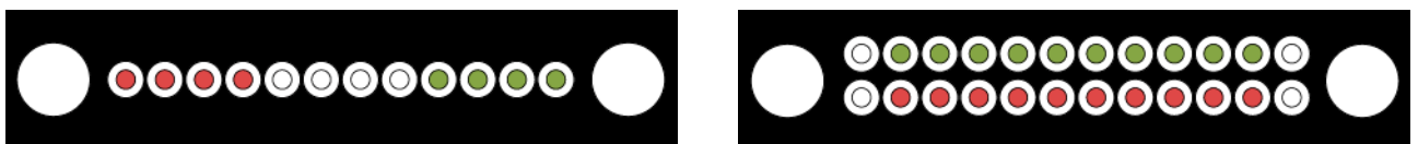
Figure 6: Diagram of MPO connectors, 12-fold (left) and 24-fold (right). The fibers for sending and receiving are color-coded, red and green, respectively.
