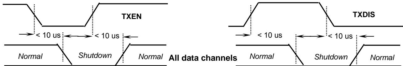
Figure 6, TXEN and TXDIS timing diagram.
