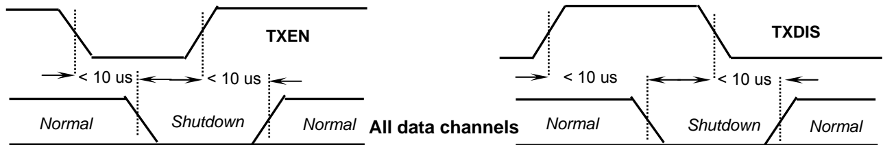
Figure 6, TXEN and TXDIS timing diagram.
