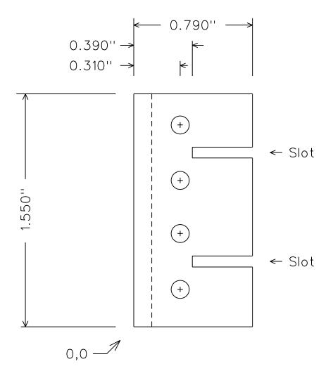
Material: hard aluminum "C" channel 0.125" thick
