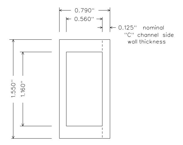
Material: hard aluminum "C" channel 0.125" thick
