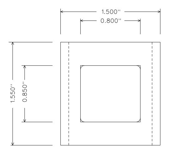
Material: hard aluminum "C" channel 0.125" thick
