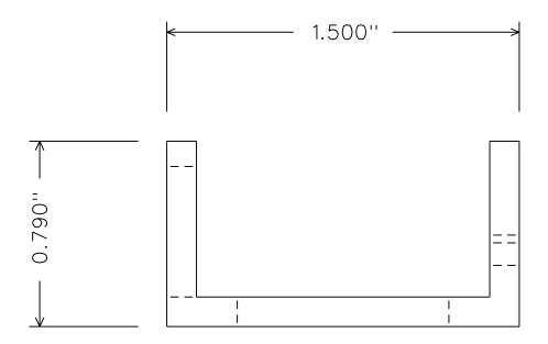
Material: hard aluminum "C" channel 0.125" thick
