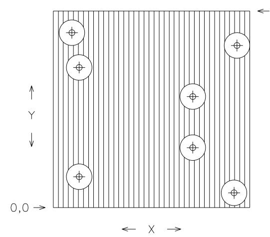
From the bar stock, cut the heatsink Y dimension to length.
